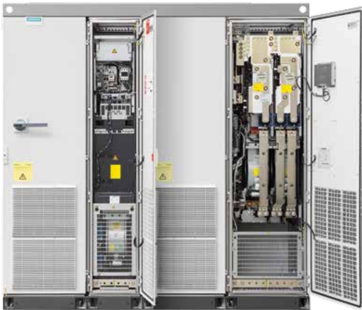
SINAMICS S150 enclosed drive 700HP with NEMA 1 filtered enclosure with transportation beams (top hats are supplied loose but not shown), 4" base (plinth)
