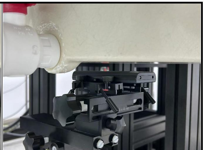
Rear Face of EUT with 1.5 cm Gap
