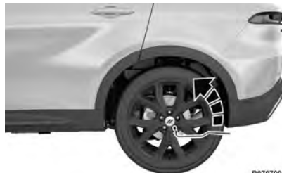
Loosening The Wheel Bolts
