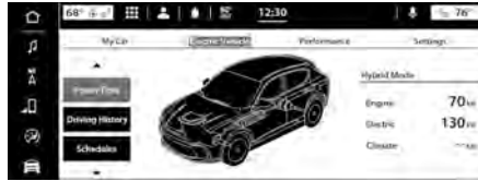
Power Flow Screen
