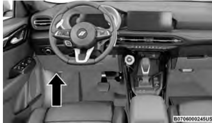
Interior Fuse Box Location
