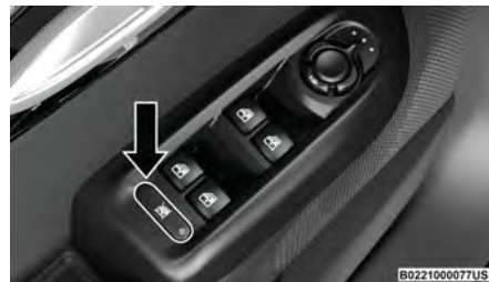
Window Lockout Switch
