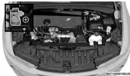
Positive (+) Battery Post
