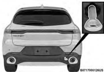
Rear Tow Eye Installed
