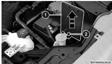
Fuse Box Cover And Locking Screw Removal
