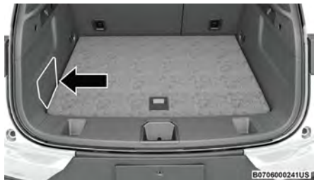
Rear Fuse Access Door Location
