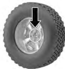
Wheel Mounting Surface
