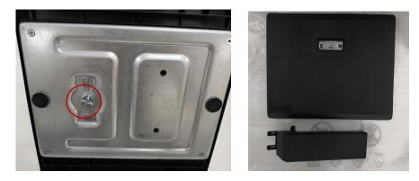
Step.14 Remove six silicon rubbers and unscrew seven screws to separate metal and plastic cover
