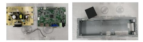
Step.9 Unscrew eleven screws and separate MID FRAME and panel
