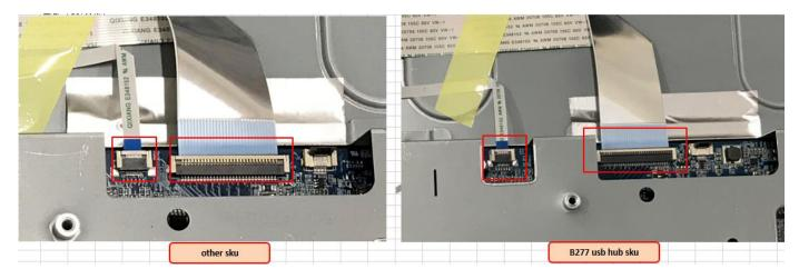
Step7. Tape AL tape to fix FFC. (Tape in red circle).
