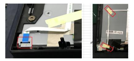
Step6. Insert 10 pin back light FFC and 30 pin LVDS FFC to main board. Use yellow tape to fix.
