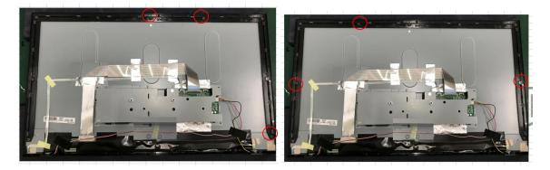
Step10. If with speaker model, assembly speaker on middle frame, and assembly speaker cable on main board. (red and white cable is on left side, yellow and black is on right side.)
