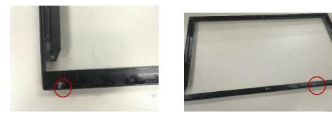
Step.11 Unscrew two screws and disassemble key board from rear cover and separate navi key& cable
