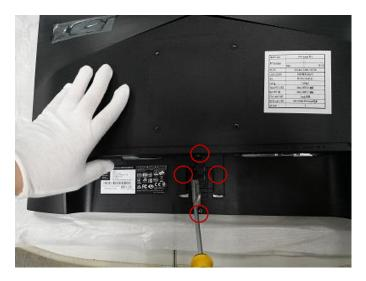
Separate hooks between MID\_FRAME and Rear cover Step.3
