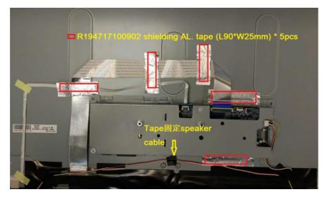
Step.6 Separate speaker from MID\_FRAME and LVDS & Backlight FFC from LCM
