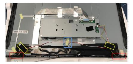
Step12. Insert key board FFC on main board, B277 with USB hub model also need to insert USB FFC on main board.
