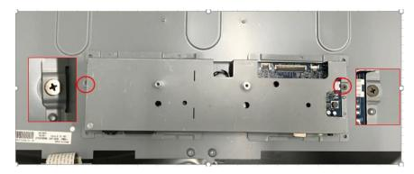
Step4. Use AI tape to fix shielding (tape in blue circle).
