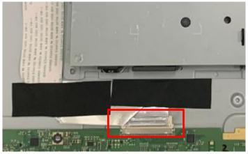
Step3. Lock the shielding on panel with screw. (in red circle)
