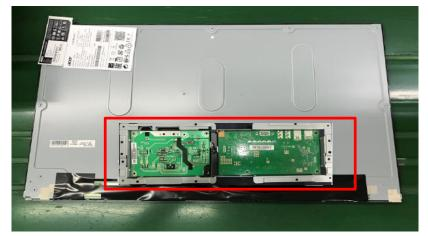
Step2. Insert 30 pin LVDS FFC to LCM, then use acetate cloth tape to tape FFC.
