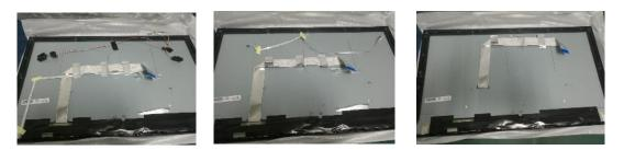
Step.7 Unscrew two hex nuts and seven screws and remove main board PCBA from main shielding.
