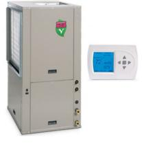
The ECO Y is a dual capacity geothermal heat pump that heats, cools, and provides a portion of a home's hot water. The communicating Premier controls work in conjunction with the dual capacity compressor and 5-speed ECM blower motor to provide comfort and savings at a great price point.
