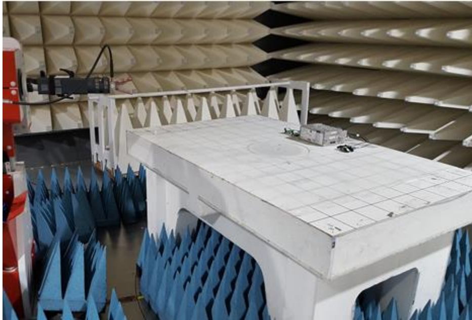
Figure C3. High Range Radiated Emission test setup 18-40GHz
