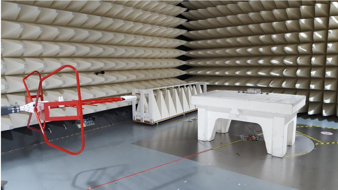
Figure C1. Low Range Radiated Emission test setup
