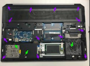
2. Remove FFC, cable, antenna & connector on chassis side: Power/TP module/Finger printer/Speaker/antenna/dream color/NFC module/smart card/cables
