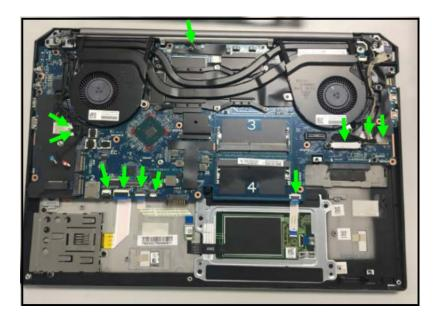
3. Remove screw\*5 to disassembly thermal fan/ Remove screw\*8 to disassembly main board
