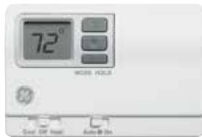
RAK164P2 (AZ 25, 28, 29, 41, 45, 75 & 85) Cooling with Electric Heat Programmable Remote Thermostat • 24V AC programmable remote wall thermostat with single-stage cooling and single-stage heating for resistance heat models • Programmable for 7-day or 5+2-day programs • Requires 5-wire hookup
