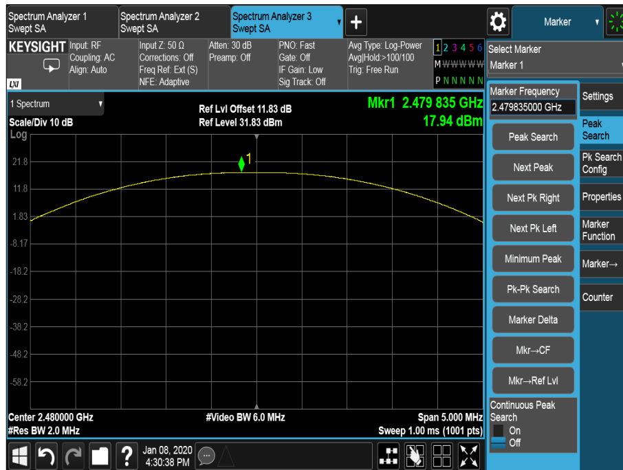
Figure 35 - 2480 MHz, GFSK - Maximum Output Power
