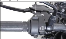
(1) Passing switch (2) Clutch switch
