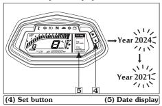
To set month, press the mode button (3) to switch from year to month display. Now press the set button (4) until the desired month is displayed.
