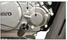
(1) Mounting bolts(2) Engine oil filter element cover
