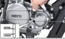
(1) Oil level dipstick (3) Lower level mark (2) Upper level mark
