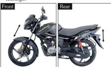
Check the rear shock absorber by pushing hard downwards on rear grip while the vehicle is not parked on stand. The suspension action should be smooth and there should be no oil leakage.
