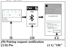
· On pairing, meter console displays "Connected" (12) below bluetooth symbol Navigation: in bluetooth mode (13).
