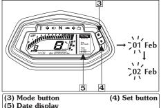
• To end the adjustment press the mode button until date display stops blinking.
