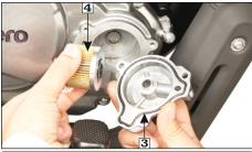
(3) O-ring (4) Engine oil filter element
