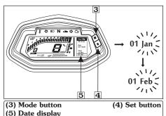
To set day, press the mode button (3) to switch from month to day display. Now press the set button (4) until the desired day is displayed.
