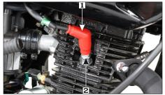
(1) Noise suppressor cap (2) Spark plug
