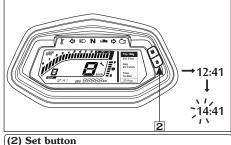
• Press the mode button (3). The minutes display starts blinking.
