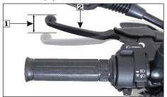
(1) Free play: 10-20 mm (2) Clutch lever (3). Turn the adjusting nut (4) to obtain the specified free play. Tighten the lock nut and check the adjustment.
