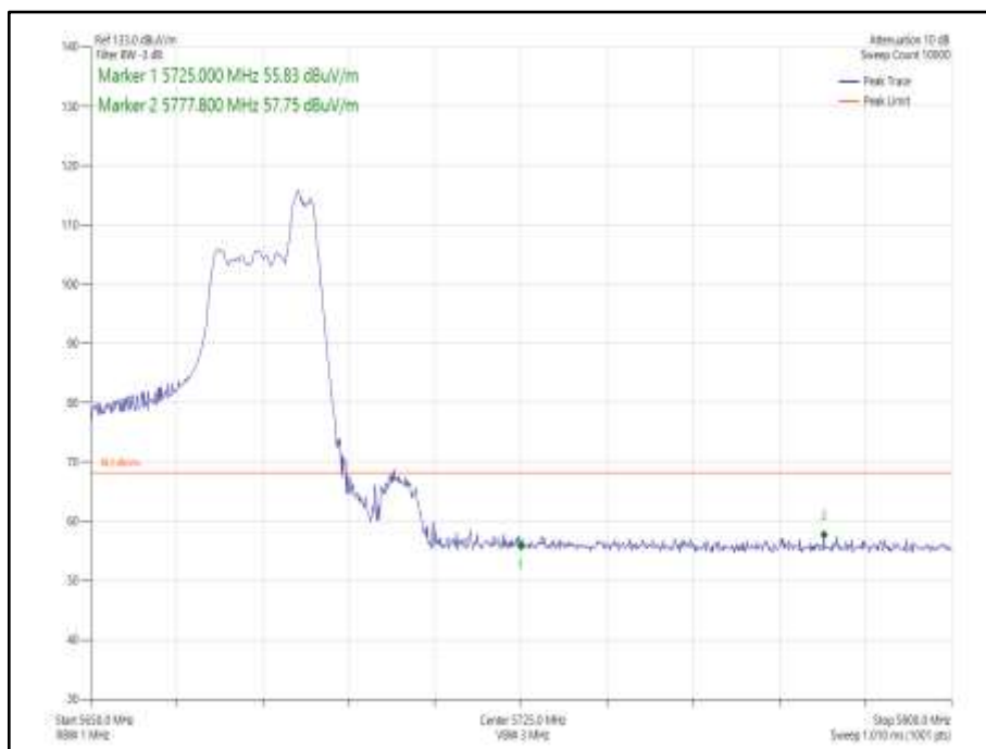
Figure 1037 - 802.11ax HE40 CDD, Cores 0-1, 52-44 - 5670 MHz Band Edge Frequency 5725 MHz
