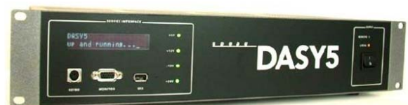
Picture C.8 Server for DASY 5
