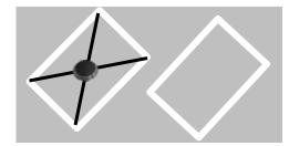
Figure 3 Determination of the center of the parking space
