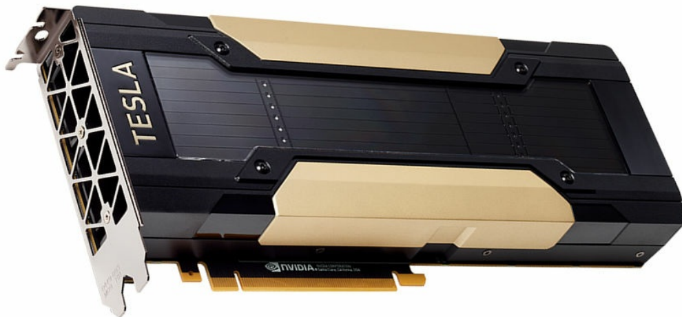
Figure 1. ThinkSystem NVIDIA Tesla V100
