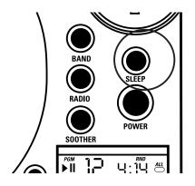
Use the sleep timer to fall asleep to the Sound Soother, radio or CD. The selected audio will automatically shut off after the programmed time.
