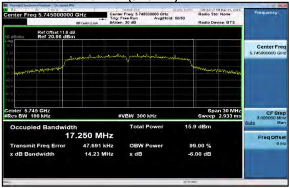
6dB Band Width Test Data CH-Mid (5785 MHz)
