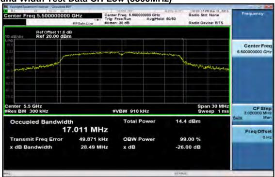
26dB Band Width Test Data CH-Mid (5580MHz)
