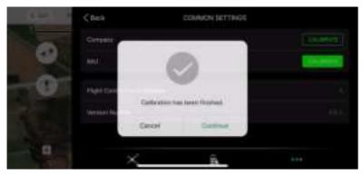
*Notice* if the SharkX appears forward or backward shift during flight, re-calibrate the compass. If problem still exists, contact local distributor/dealer and seek help.
