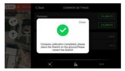
Notice calibrate the compass when there are no less than 15 satellites
