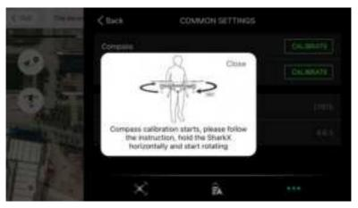
4.5.4. Following the audio instructions, hold the drone horizontally with its nose outwards and complete the horizontal calibration. And then hold the drone vertically with its nose downwards and complete the compass calibration.
