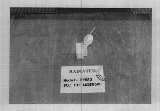
3.4 Radiated Emission Configuration Photograph (cont.) - Handset
