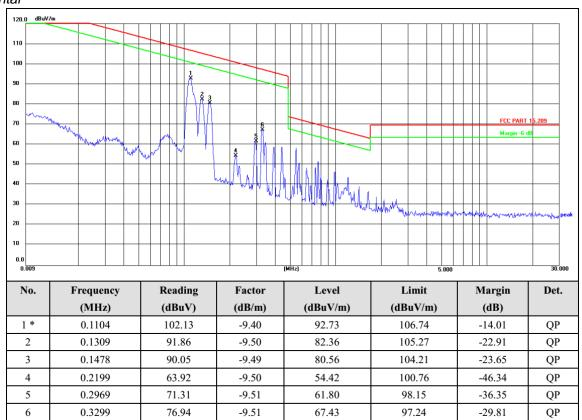
Remark: 1). Measured at antenna position 0 degree and 90 degree, recorded worst case at 0 degree.
