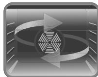
This function is good for baking pastry. Cooking is carried out by the lower and upper heating elements within the oven and by the fan, which provides air circulation, giving a slightly grilled effect to the food. It is recommended that you preheat the oven for about 10 minutes. The fan and lower heating function is ideal for baking food, such as pizza, evenly in a short period of time. The fan evenly disperses the heat of the oven, while the lower heating element bakes the food.
