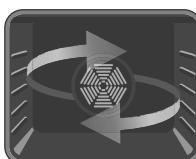
**Defrost Function:** The oven's warning lights will switch on and the fan will start operating. To use the defrost function, place your frozen food in the oven on a shelf placed in the third slot from the bottom. It is recommended that you place an oven tray under the defrosting food to collect the water from melting ice. This function will not cook or bake your food, it will only help to defrost it.
