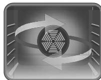
is ideal for baking food, such as pizza, evenly in a short time. The fan evenly disperses the heat in the oven, while the lower heating element ensures baking of the food.
