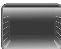
**Static Cooking Function:** The oven's thermostat and warning lights will switch on, and the lower and upper heating elements will start operating. The static cooking function emits heat, ensuring
