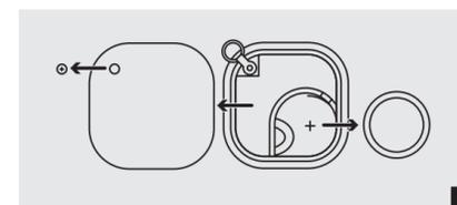
If the item locator is not working, you may need to replace the battery. Use a screwdriver to remove the screw and open the battery back cover and remove the old battery.
