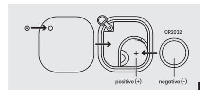
Insert the new battery in the proper direction as indicated by the positive (+) and negative (-) symbols and replace the battery back cover and tighten the screw.
