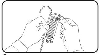
3 Peel off backing to expose adhesive tape and stick LED modules into place.
