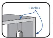
A 2 in. (51 mm) border is recommended along the perimeter of the sign.
