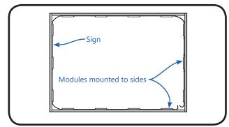
Determine location of where LED modules will be mounted based on sign dimensions (see chart on page 4). If mounting on bottom of sign, the use of a riser will be needed (minimum 1/8 in. distance between bottom surface and module).
