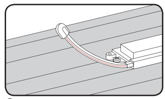
Cap all exposed wires with appropriate end caps or apply electric grade (non-conductive) silicone for additional weather protection.
