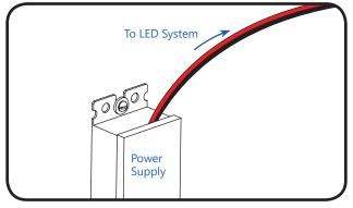
3 Run a wire from the Power Supply and connect to the first LED module on the strip.
