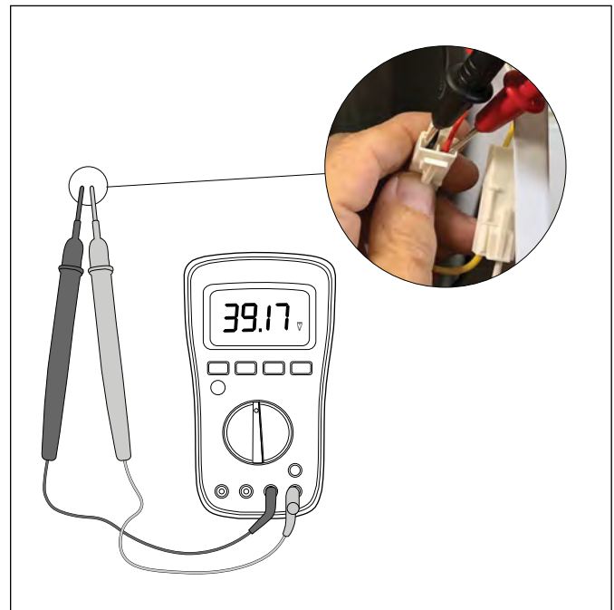
Figure 8 Applied Voltage Measurement Method
