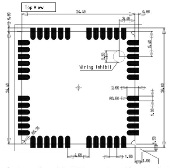
In order to easily rework the GE868 is suggested to consider on the application a 1.5 mm placement inhibit area around the module.
