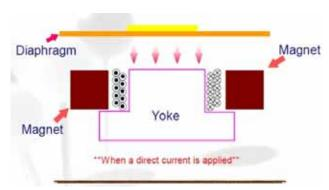
Drawing of the Magnetic Buzzer.
