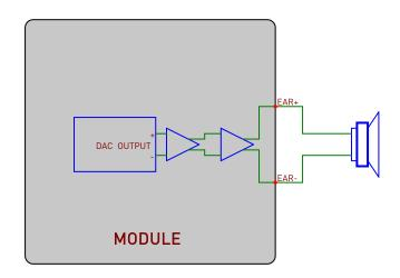
The audio output of the GL868 is balanced, this is helpful to double the level and to reject common mode (click and pop are common mode and therefore rejected). These outputs can drive directly a small loudspeaker with electrical impedance not lower than 80hm.
