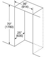
Leave 1/2" (12.7) gap at the top and 1" (25.4) behind the refrigerator for proper ventilation. It is recommended that you do not install the refrigerator near a heat source such
