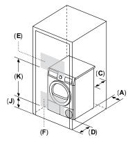
Minimum clearance requirements (Stacked, Stand Alone or Side by Side): A: Both sides (left and right) – 5/8"
