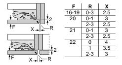
The gap dimensions recommended in the table must be maintained to guarantee collision-free opening of appliance doors and avoid damage to kitchen furniture.
