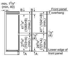
The specified unit door dimensions are valid for a door gap of <sup>1</sup>/8" (4 mm).
