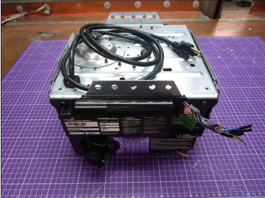
Above Antenna Ports populated in final product. Pictured below is the complete GDO that the Phoenix Logic Board will sit inside.
