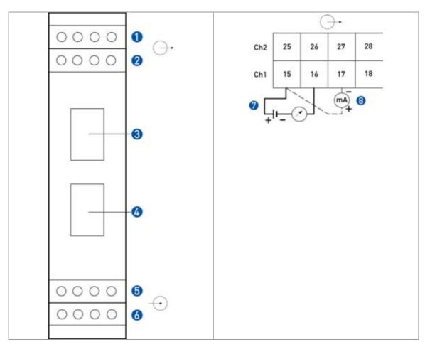
Figure 3: TT 31 R connection diagram
