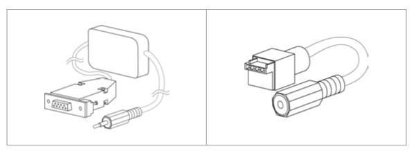
Figure 7: PC connection cable
