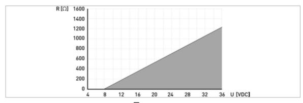
Figure 8: Output load diagram TT 31 R, TT 31 R
