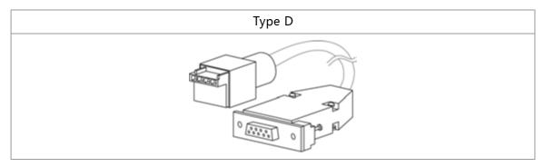
Figure 5: PC connection cable (offline cable)
