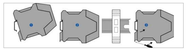
Figure 1: Rail installation
