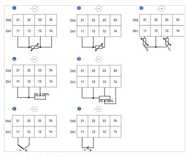
Figure 2: Installation diagram TT 31 R
