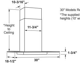
30" Models Require a 30"-Wide Opening \*The supplied duct cover fits 7'-5" to 9'-3" ceiling heights (10' with optional high ceiling kit JXDC71)
