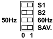
Figure 7. SE series DIP switch
