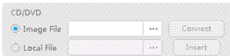
Figure 3-43 Mounting a DVD-ROM drive
