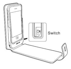
3.Connect to USB power adapter (excluded) with included USB cable to charge\_\_\_ the Power Case.
