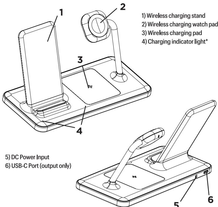
\*A blinking amber LED indicates a foreign object has been detected (metal objects like keys, coins, etc.) and the device is automatically turned off to ensure safety. Removal of the foreign object and proper alignment of phone will result in normal operation.
