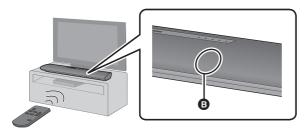
B Remote control signal sensor
