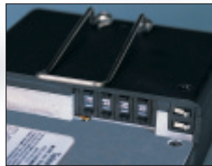
Code Switch: Allows operator to select up to 65,000 different cipher codes (BTR-600 set only).
