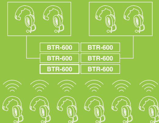
6 "drop" system interfaced into wired party line intercom
