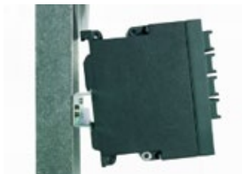
Figure 4-2 Removing from a 35 mm DIN rail
