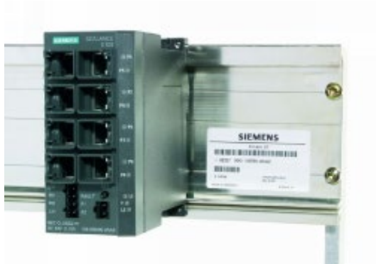
Figure 4-3 Installation on a SIMATIC S7-300 standard rail
