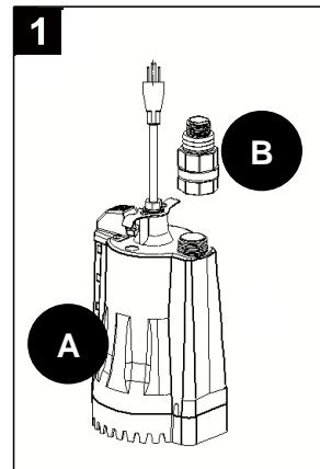
2. Connect either a 3/4 in. garden hose to the threads of the adaptor (B) or clamp a 1-1/4 in. hose kit (Item #0313726, sold separately) to the barbs of the adaptor (B).
