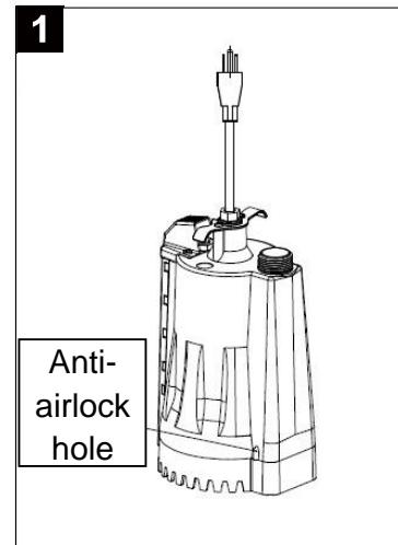
**CAUTION: This hole is for anti-airlock purposes. Leakage of air or water is NORMAL. DO NOT BLOCK THIS HOLE!**
