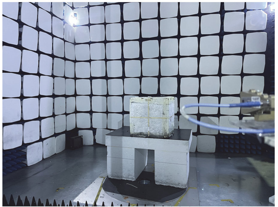
Radiation Emission Test Setup (Above 18GHz)
