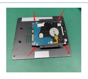
3. Tighten the screws on both sides. (Four in total)
