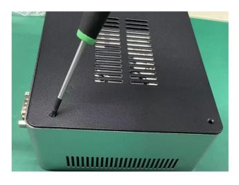
2.Use a screwdriver to unscrew the screws to open the bottom case.
