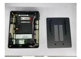
3.after open the bottom case, you will see inside slot for RAM SSD and header on the motherboard
