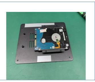
2. Align the drive with the bracket screw holes.
