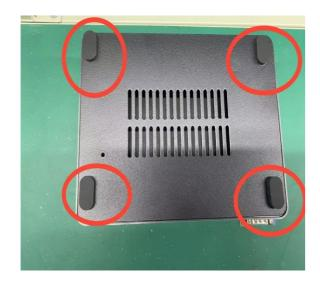
1.To remove the bottom case, first remove the four foot cover.
