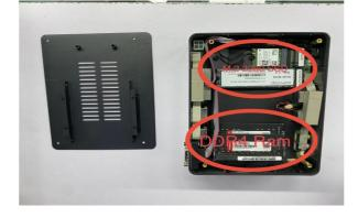
4. The memory and SSD are installed in the locations shown in the photos. SSD support 2 slot for NVME/SSD & ONLY NVME SSD
