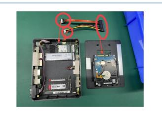
4.Connect the hard drive to the motherboard connectors with the attached special SATA cable and SATA power cable.
