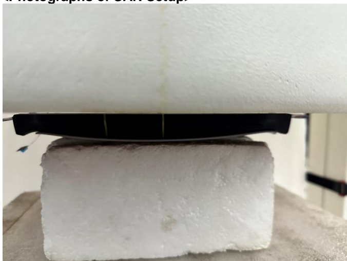
Fig-4.1 Front Face of EUT with 0 cm Gap (Extremity Mode)
