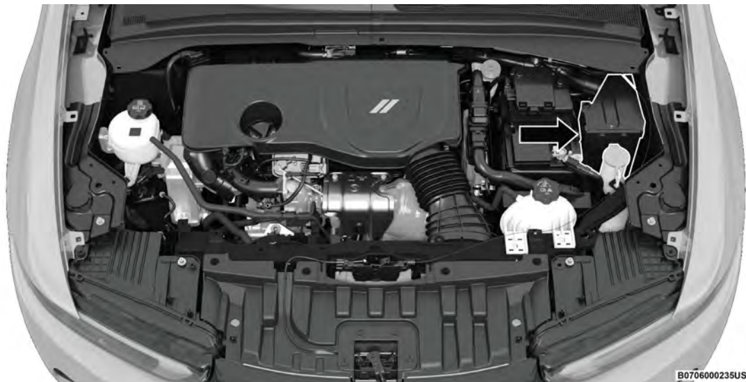
Underhood Power Distribution Location
