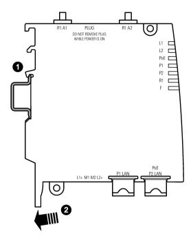
Follow the steps below to fit the SCALANCE W774/W734 to a DIN rail:
