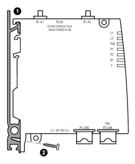
Follow the steps below to fit the SCALANCE W774/W734 to an S7-1500 standard rail:
