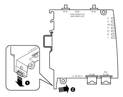
Follow the steps below to remove the SCALANCE W774/W734 from a DIN rail:
