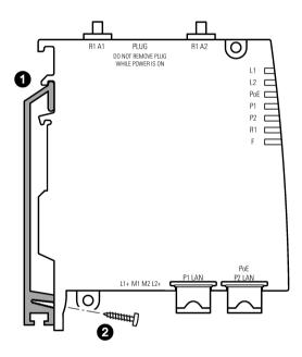
Follow the steps below to fit the SCALANCE W774/W734 to an S7-300 standard rail:
