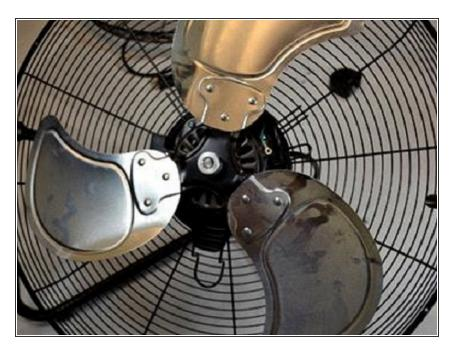
Remove the green wire that is attached to the motor housing.
