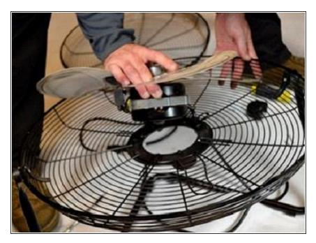
Remove the motor from the back of the fan cover.
