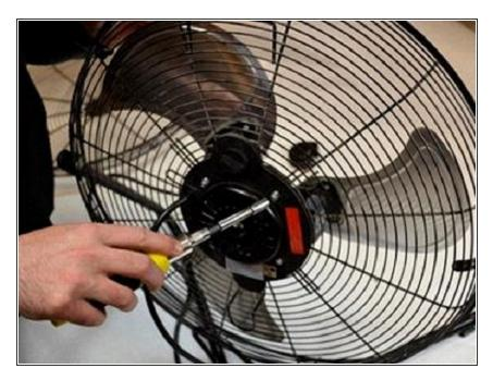
Remove the nuts securing the motor to the back cover of the fan, using a Phillips #2 screwdriver and an 8mm socket driver.
