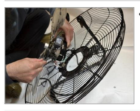
The fan is fully disassembled; replace the damaged parts.
