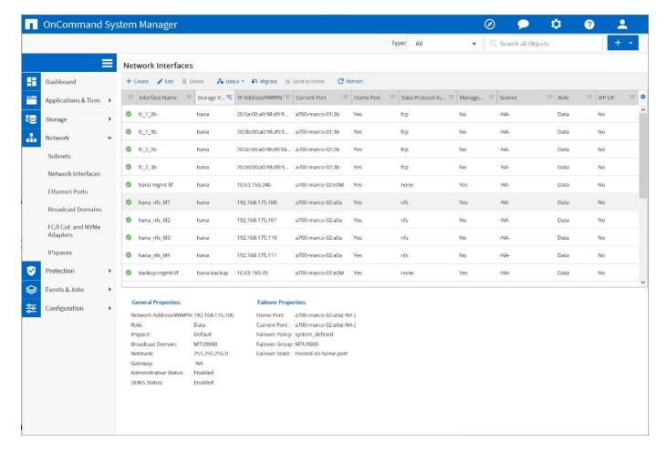
During SVM creation with ONTAP 9.8 System Manager, all the required physical FCP ports can be selected, and one LIF per physical port is created automatically.
