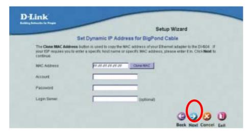
address, please enter it in. The CLONE MAC Address button is used to copy the MAC address of your Ethernet adapter to the DI-604 WAN interface. Click **Next**
