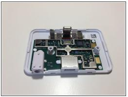
• Remove the two screws that secure the weight to the plastic housing.
