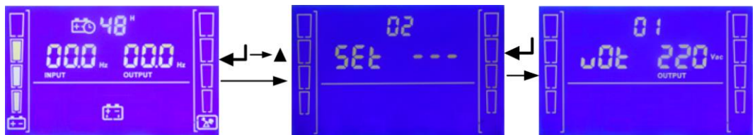
Figure 5-10 Setting the voltage level
