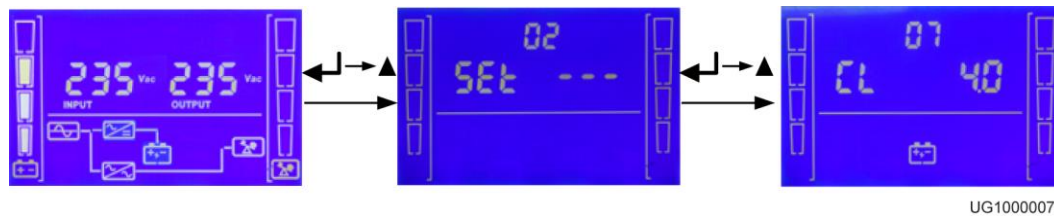
Figure 5-6 Setting the charge current limit
