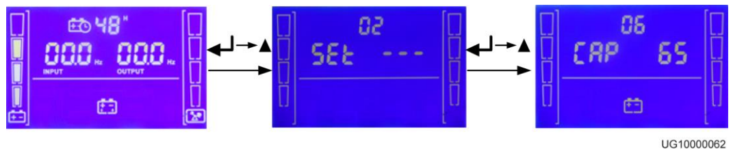
Figure 5-13 Setting the battery capacity
