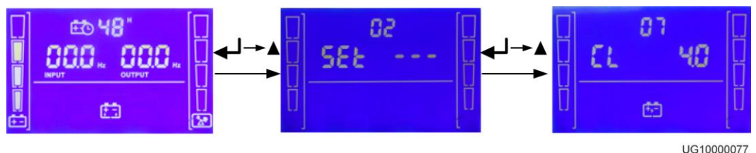
Figure 5-14 Setting the charge current limit
