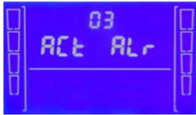
Figure 4-7 Active alarm display menu
