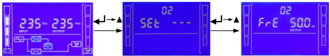
Figure 5-3 Setting the output frequency level
