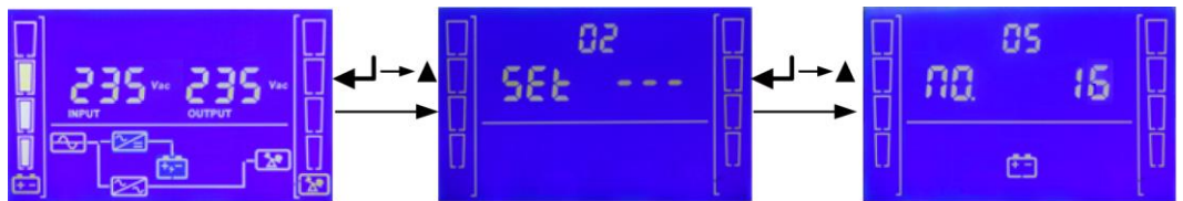
Figure 5-4 Setting the number of batteries
