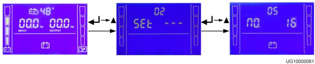
Figure 5-12 Setting the number of batteries
