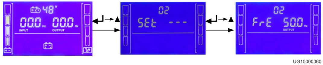
Figure 5-11 Setting the voltage and frequency
