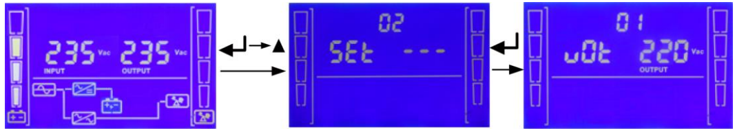
Figure 5-2 Setting the voltage level
