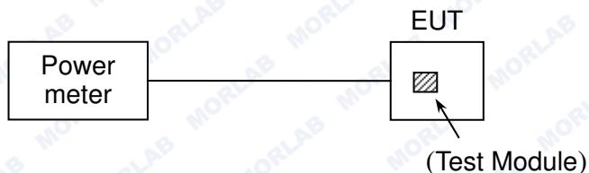
The EUT (Equipment under the test) which is powered by the Battery is coupled to the Power Meter; the RF load attached to the EUT antenna terminal is 50Ohm; the path loss as the factor is calibrated to correct the reading, all test result in power meter.
