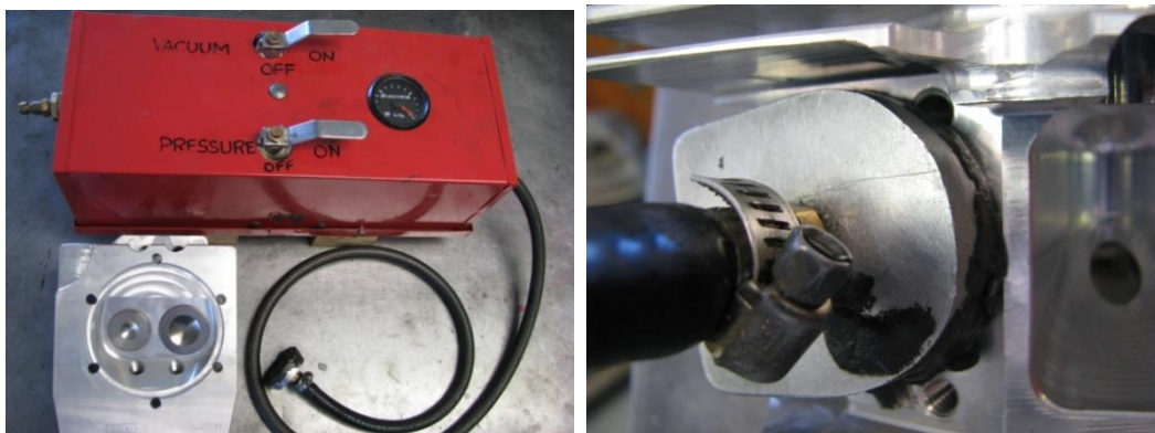
Figure 18 – Valve Leakage Vacuum Tester
