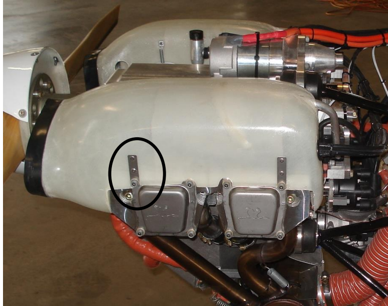
Figure 32 – Air Duct Hard Point Reinforcement
