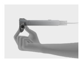
**CAUTION:** To replace Nose Pad, grip between fingers and pull straight out of headset, not down.
