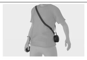
Clip the Shoulder Strap hooks to the Compute Pack posts. Wear the strap over your shoulder, just like a messenger bag. Adjust the strap length for optimal positioning and comfort.
