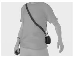
Clip the Shoulder Strap hooks to the Compute Pack posts. Wear the strap over your shoulder, just like a messenger bag. Adjust the strap length for optimal positioning and comfort.
