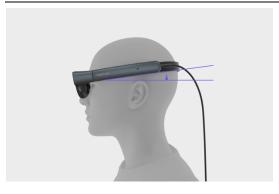
To find the right viewing angle, raise or lower the Headset until you can see all 4 corners of the animation at the same time. Then secure in position by pushing the Back Band together.
