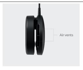
**CAUTION:** Do not block the Compute Pack air intake or air exhaust while in use.
