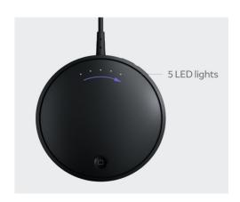
Press and hold the power button on the Compute Pack until the LED lights begin to illuminate.
