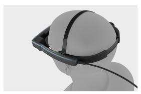
Place the Headset back on your head, continue adjusting the Overhead Strap until it's secure and comfortable, then fasten the velcro.
