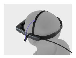
If the back of the Headset slips while wearing the device, simply add the Overhead Strap.
