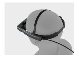
Place the Headset back on your head, continue adjusting the Overhead Strap until it's secure and comfortable, then fasten the velcro.
