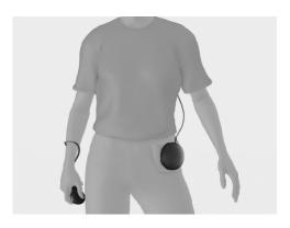
With the Power button on the outside, slide the back-half of the Compute Pack into a pocket or waistband until it's fixed and secure.
