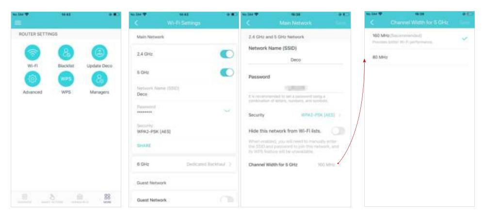
6 GHz Wi-Fi is used for dedicated backhaul by default. When it is used for your Wi-Fi network connection, you can change your 6 GHz network's Wi-Fi name and password, hide the network from Wi-Fi list, etc. Only Wi-Fi 6E-compatible devices can search for and join the 6GHz nework.
