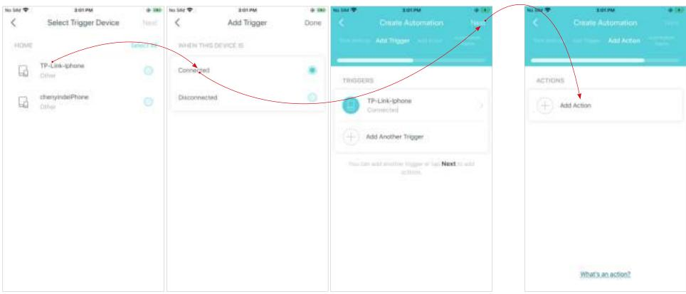
5. Select the trigger device and set the trigger details.
